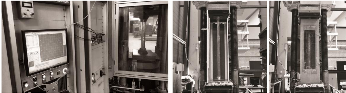
Figure 5. Left: Experimental set-up of the 0.5 m high specimens. Centre and right: Experimental set-up of the 1.5 m high specimens.
