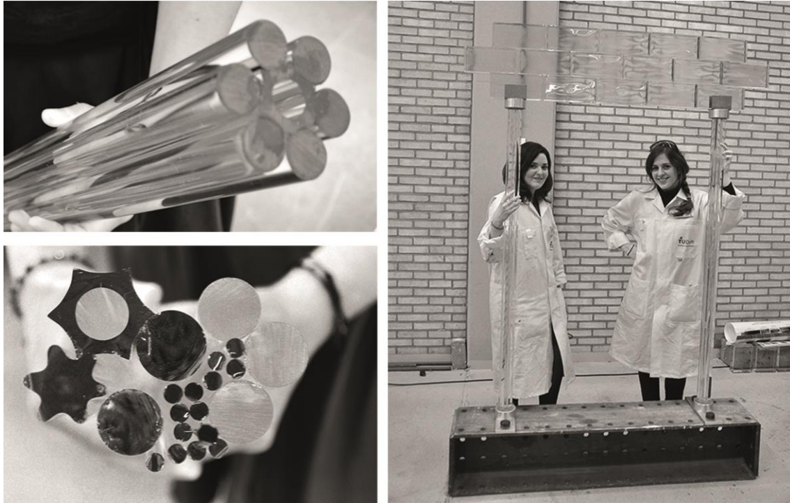
Figure 4. Top Left: Concluded configuration of the bundled glass column. Bottom Left: CONTURAX ® and DURAX ® profiles. Right: Realized 1.5 m high prototypes.
