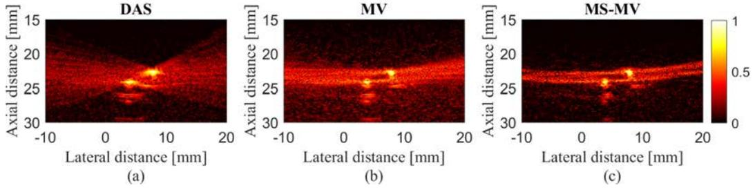
Fig. 1. The reconstructed experimental PA images using (a) DAS, (b) MV and (c) MS-MV. All the images are shown with a dynamic range of 50 dB. Two wires are used as the imaging target.
