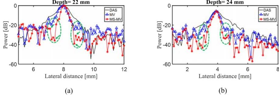
Fig. 2. The lateral variations of the reconstructed PA images shown in Fig. 1. Arrows and circles demonstrate the improvement caused by MS-MV algorithm.
