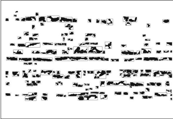
Fig. 4 Bounding boxes taken to be the rectangles around the observable 2D features of interest in the microstructure. Sample size is n = 175
