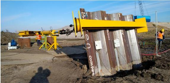
Figure 4. Photo of AZ13-700 during the test
