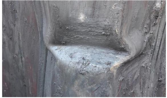
Figure 14. Excavated GU8N-rev with local buckling
