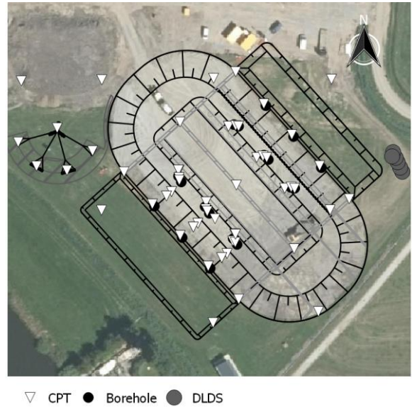
Figure 1 Topview FST site with soil investigation points.
