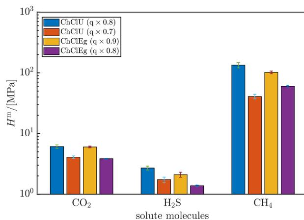
**Fig. 5.** Comparison of the computed Henry constants (molality based) of CO<sub>2</sub>, H<sub>2</sub>S, and CH<sub>4</sub> in ChClU and ChClEg DESs, using the GAFF force field parameters with different ionic charge scaling factors for the DESs.
