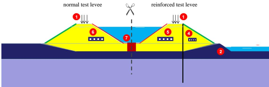
Figure 2: Cross section test levee without (left) and with (right) sheet pile wall with load (1), excavation (2), infiltration/drainage utilities (4, 5 and 6) en clay cut off wall (7)
