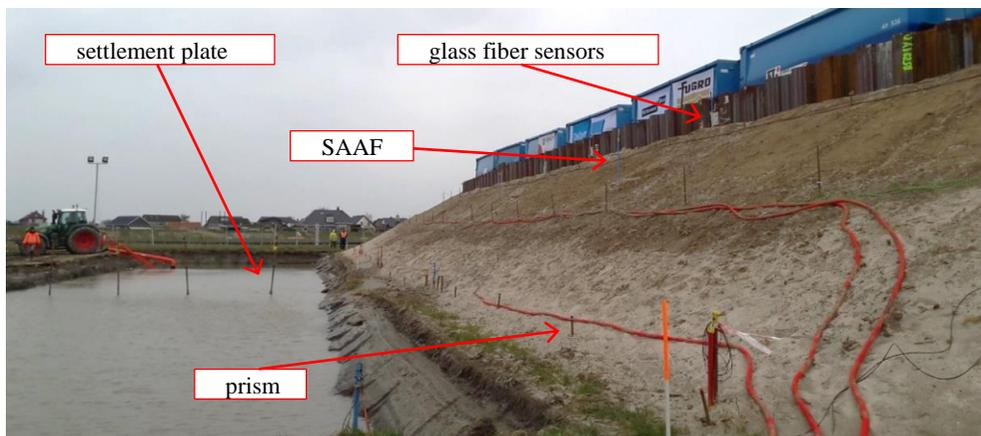
Figure 7: Monitoring campaign FST on (non-)reinforced test levee
