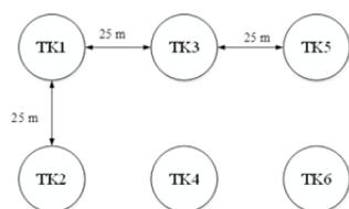
Figure 3: Layout of the gasoline tanks
