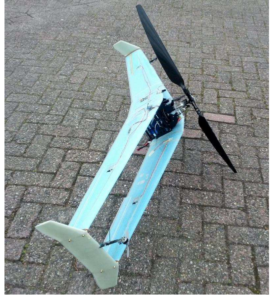
Figure 1: Novel hybrid Unmanned Air Vehicle featuring a cyclic controlled rotor with wing.
