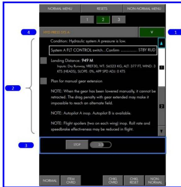
**Fig. 1** By pressing the arrow on the right-hand side (1), the dropdown menu can be opened and closed. The dropdown menu itself consists of the reduced checklist content (2) and a row from which automation and checklist progress is controlled and supervised (3). When deemed necessary, the complete checklist can be accessed by pressing the checklist name (4), alike on the Boeing 787 ECL
