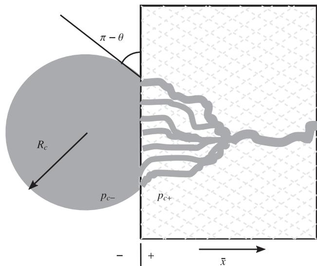
**Figure B-1.** Schematic of a potential transition region near a droplet (or bubble, in which case  $\pi - \theta$  becomes  $\theta$ ) the flow channel, we assume any deviation from one-dimensionality to be negligible. The “-” and “+” are denoted in the figure. The contact angle is denoted as  $\theta$  and the radius of curvature of bubble/droplet is denoted as  $R_c$ .
