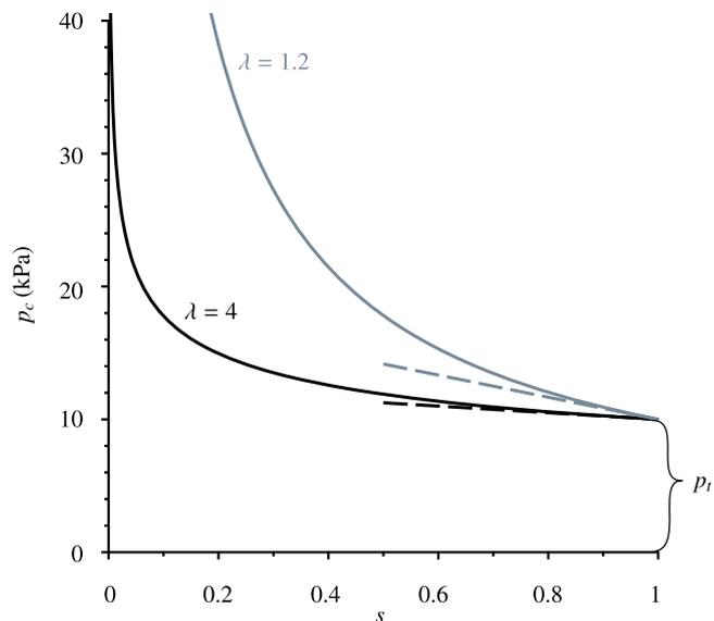
**Figure 2.** Capillary pressure curves for different pore size distribution index  $\lambda$  for  $p_t = 10$  kPa. The dashed lines show the linearization  $p_c = p_t \frac{1+\lambda-s}{\lambda}$  near  $s = 1$  for the two different values of  $\lambda$ .
