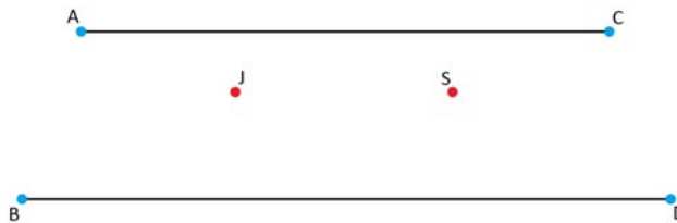
Figure 4: By locating J and S, a formation flight route is obtained for the solo routes AC and BD
