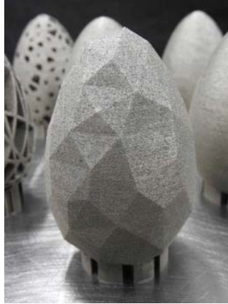
Figure 12: A sample made using Renishaw strategy illustrating a uniform surface
