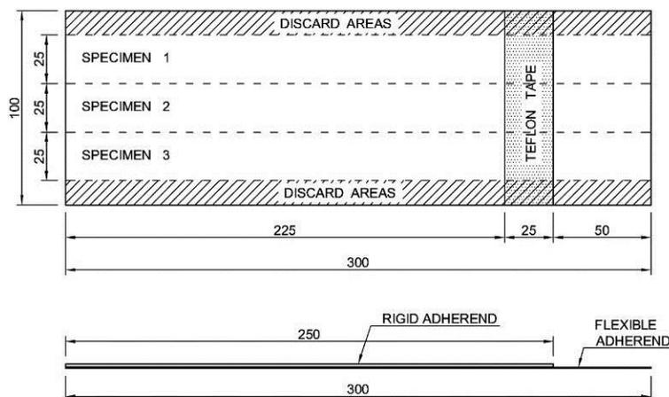
Figure 1. Bonded test panel (dimensions in mm) [3].
