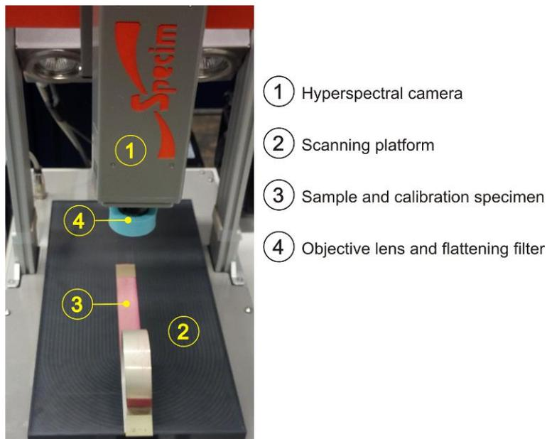
Figure 3. Photo of the laboratory hyperspectral imaging setup.
