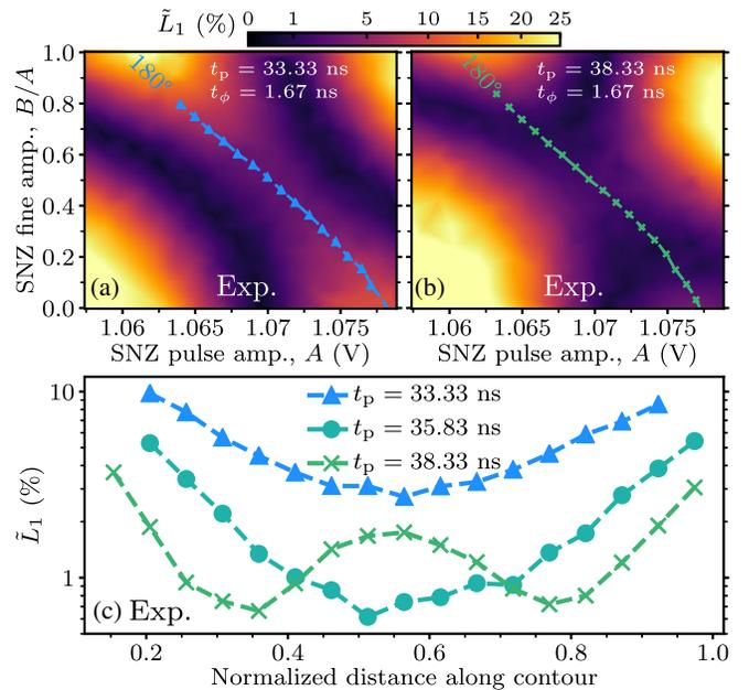
FIG. 3. (a),(b) Landscapes of the leakage estimate  $\tilde{L}_1$  for intentionally short and long SNZ half pulses on  $Q_{M2}$ . (c) Extracted  $\tilde{L}_1$  along the  $\phi_{2Q} = 180^\circ$  contours from (a),(b), and Fig. 2(c).
