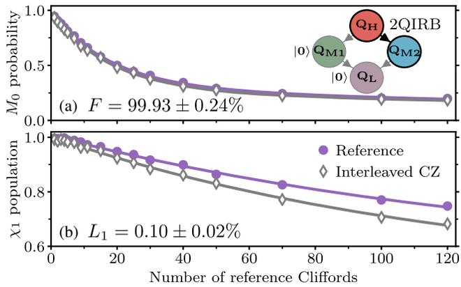
FIG. 4. Best SNZ CZ gate performance achieved from a single run of 2QIRB. (a) Reference and CZ-interleaved return probability  $M_0$  to  $|00\rangle$  and (b) population in the computational space  $\chi_1$  as a function of the number of two-qubit Cliffords in the reference curve. Errors bars in  $F$  and  $L_1$  are obtained from the uncertainty of exponential-decay fits.
