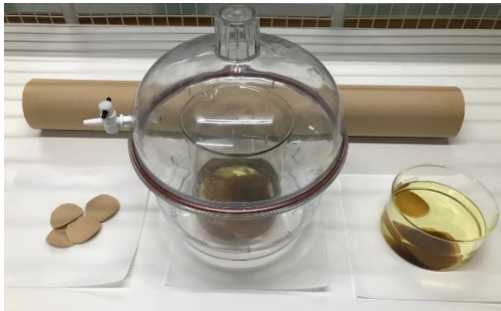
Fig. 1. Sample preparation. Paper roll, small circular paper samples, OIP samples stored inside a closed desiccator, OIP samples transferred to another glass container to be used for the test.
