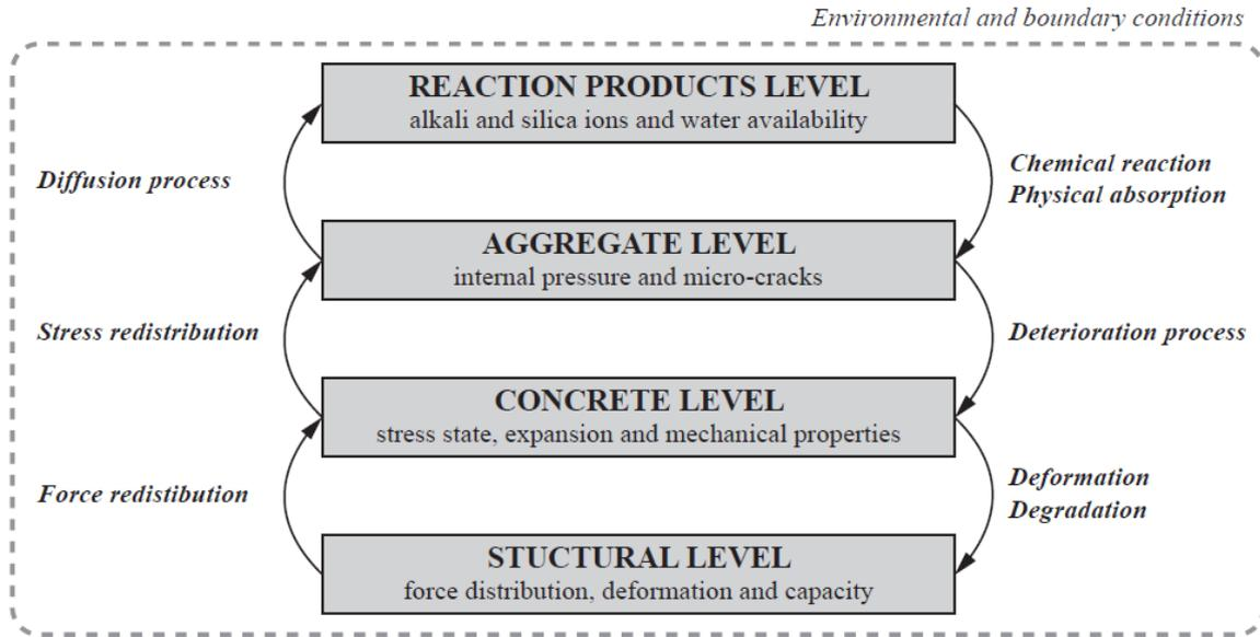
Figure 1: The alkali-silica reaction in concrete structures: interaction of the various phenomena at the different scales (Esposito, 2016).
