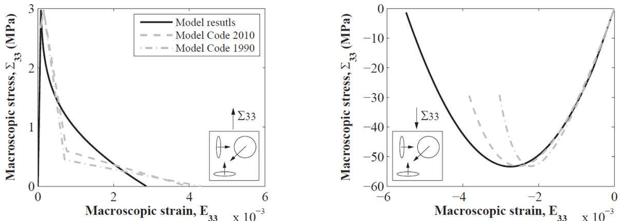
Figure 4: Simulation results of the micro-poro-fracture-mechanical model: resulting uniaxial tension softening and compression hardening-softening behaviour (Esposito and Hendriks, 2015).
