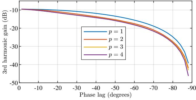
Fig. 3: 3<sup>rd</sup> order harmonic gain at  $\omega = 100$  rad/s of various  $p$  values, for different provided phase lag.
