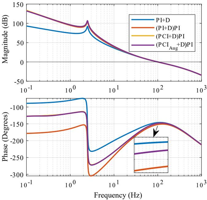
Fig. 9: Open loop frequency response of control scheme in Fig. 8. The gain and phase response of (PCI+D)PI (yellow) is below that of (PCI<sub>Aug</sub>+D)PI (purple).
