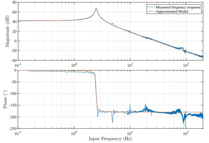
Fig. 7: Identified frequency response of the stage.
