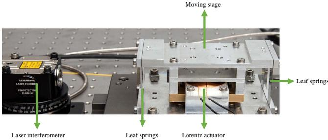
Fig. 6: The custom-designed precision stage used for experiments.
