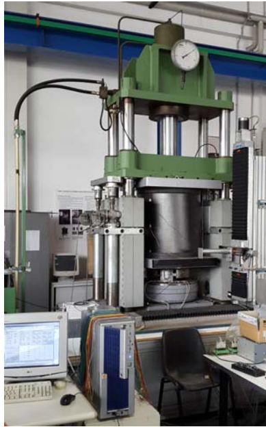
Figure 8. Buckling testing equipment.
