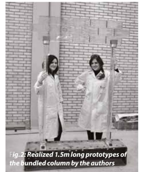
Fig.2: Realized 1.5m long prototypes of the bundled column by the authors
