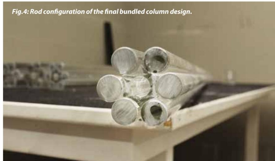
**Fig.4: Rod configuration of the final bundled column design.**
