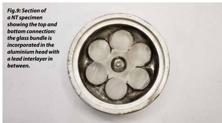
**Fig.9: Section of a NT specimen showing the top and bottom connection: the glass bundle is incorporated in the aluminium head with a lead interlayer in between.**
