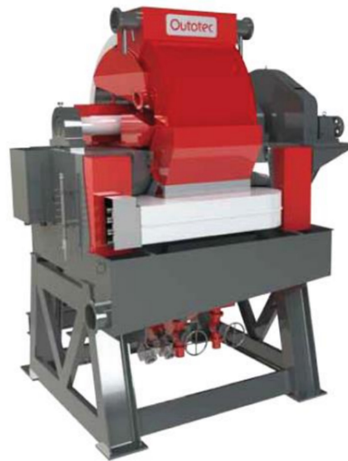
Figure 8-5: SLon® vertically pulsating high-gradient magnetic separator from Outotec.
