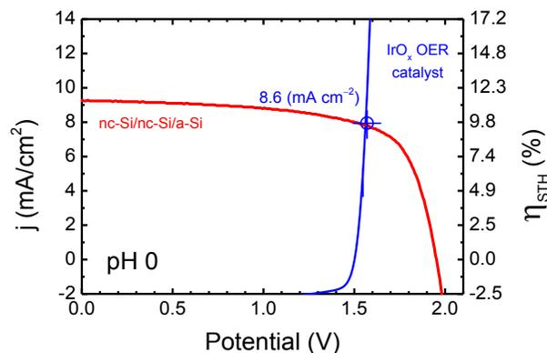
Fig. 6. JV characteristic measured as a PEC and solid state device of an a-Si:H/nc-Si:H/nc-Si:H solar cell in comparison to an IrO<sub>x</sub> counter electrode in pH 0, and the equivalent STH efficiency in which these currents translate.
