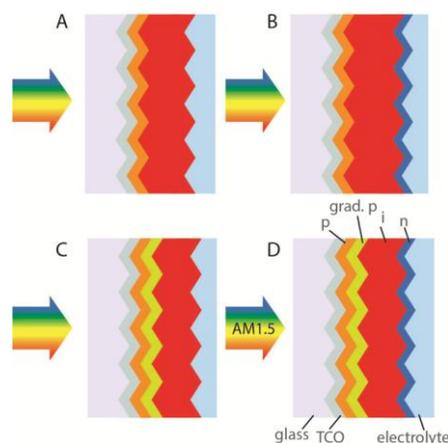
Fig. 3. Schematic illustration and PEC results of the p-i a-SiC:H photocathode (A) p-i-n photocathode (B), p-grad. p-i photocathode (C) and p-grad. p-i-n photocathode (D).
