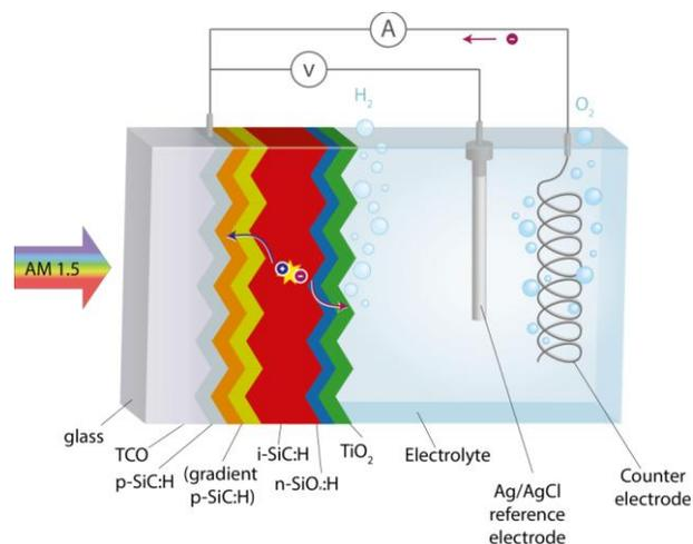
Figure 1. Schematic representation of the 3-electrode photocathode configuration
