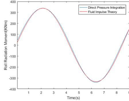
(b) Comparison of Fluid Impulse Theory(FIT) and the Direct Pressure Integration(DPI) results for roll amplitude of 0.05rads at roll natural frequency(0.76rad/s)
