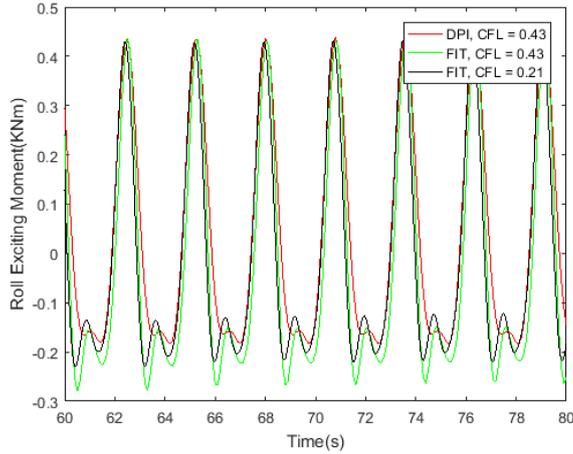
Figure 2: Roll exciting moments on barge of beam  $B=12\text{m}$  and draft  $T=2.4\text{m}$  by waves of waveheight of  $0.1\text{m}$  and the wavelength  $12\text{m}$
