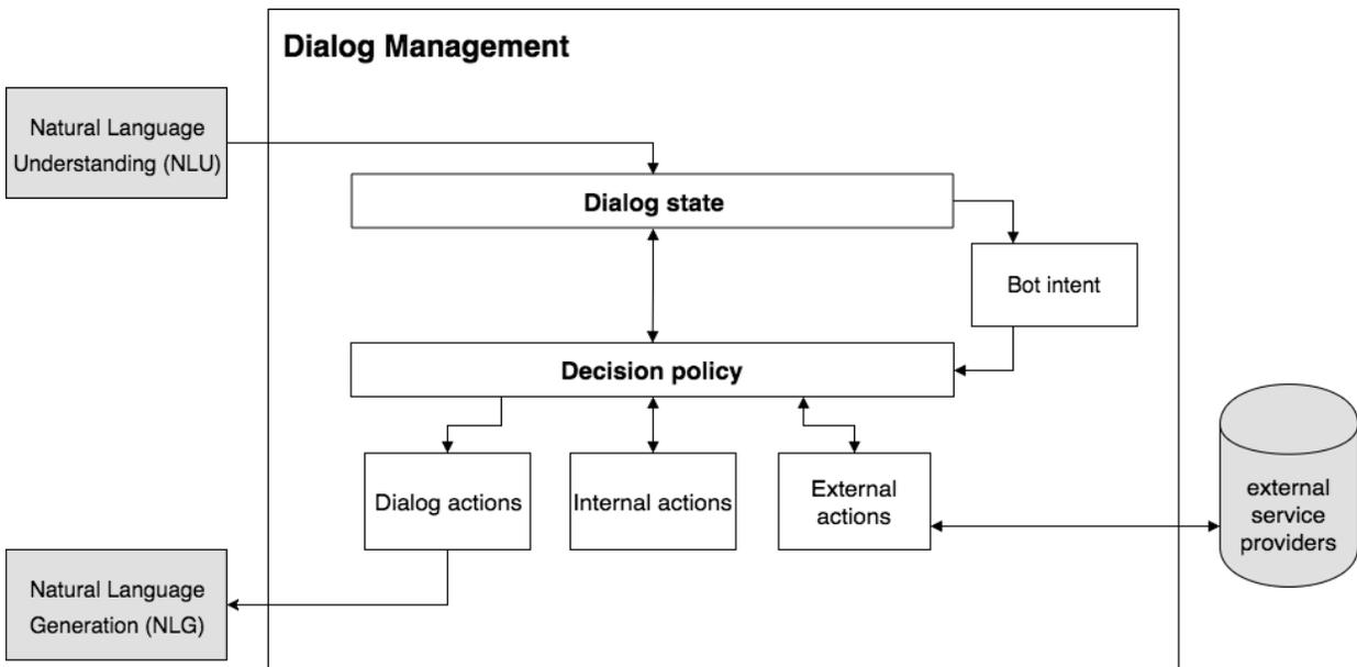
Figure 1 - Dialog management system architecture and information flow
