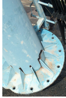
Fig. 2. Detail of the rupture at mid-height
