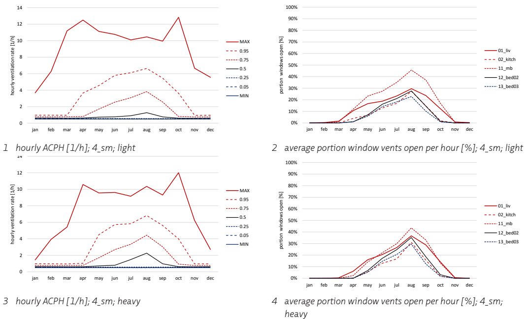
FIGURE 6.11 Percentiles of hourly ACPH [1/h] for the whole house and portion of opening of the window vents [%] per room for the variant with adaptive control of ventilation for temperature; occupancy profile 4_sm
