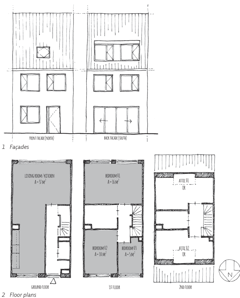
FIGURE APP.D.1 Façades and floor plans of the reference dwelling of AgentschapNL used in the TRNSYS calculations
