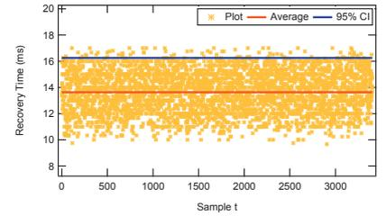
Fig. 6: Recovery times for 5 ms transmit interval in the extended topology.
