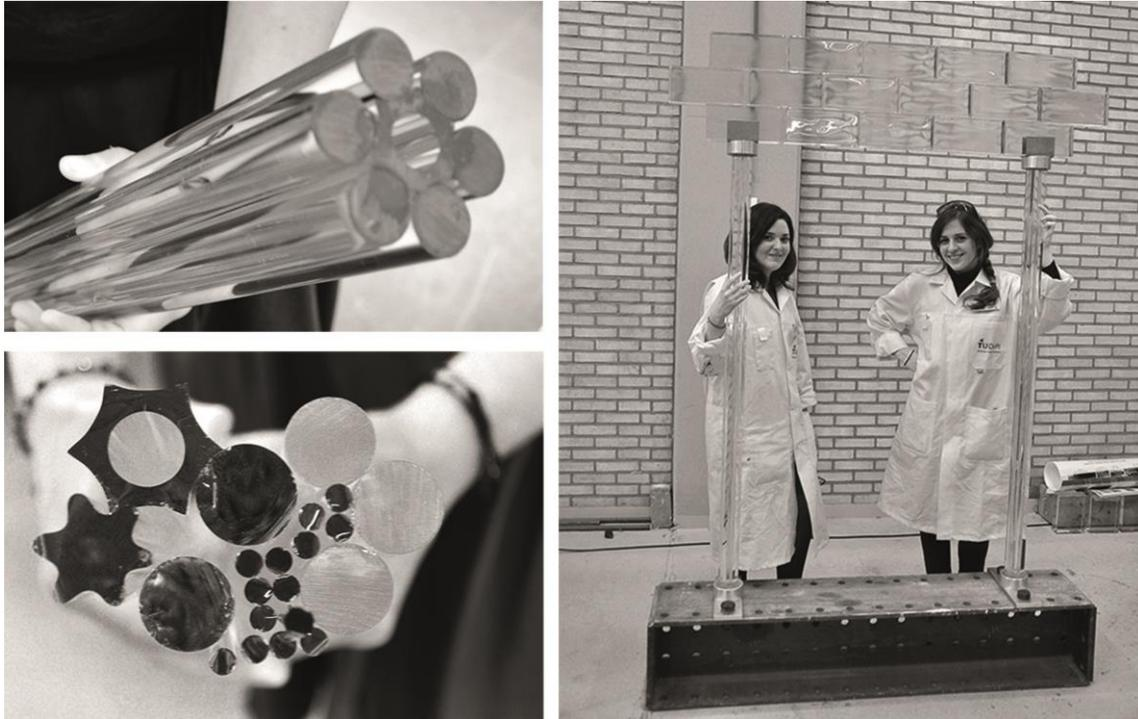
Figure 4. Top Left: Concluded configuration of the bundled glass column. Bottom Left: CONTURAX<sup>®</sup> and DURAX<sup>®</sup> profiles. Right: Realized 1.5 m high prototypes.
