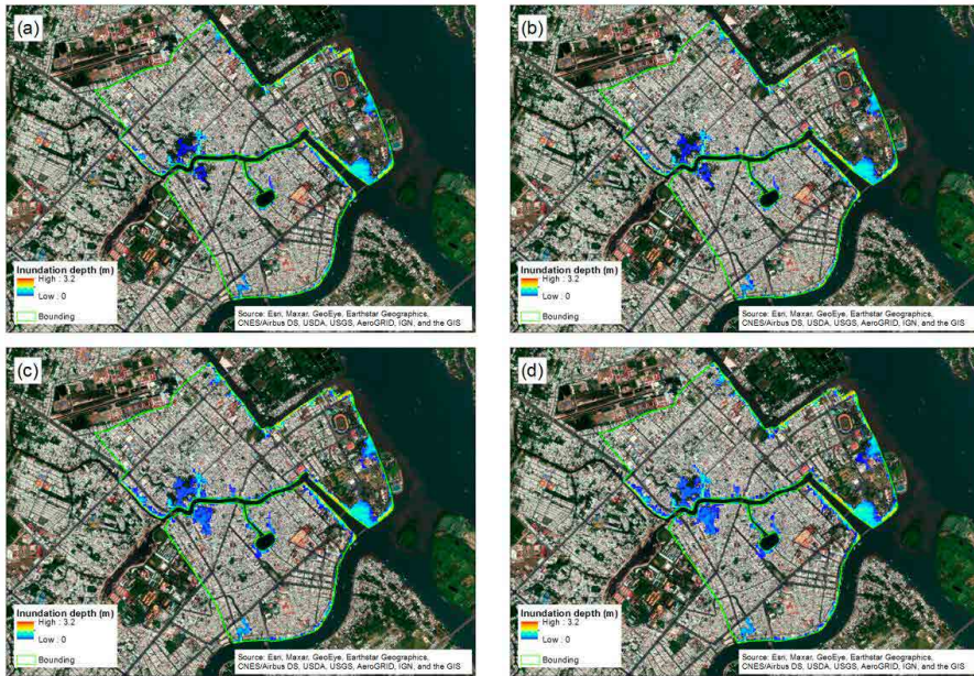
Figure A.1. Flood hazard maps for the present corresponding to each return period of water level, (a) 1 yr return period, (b) 2 yr return period, (c) 10 yr return period, (d) 20 yr return period
