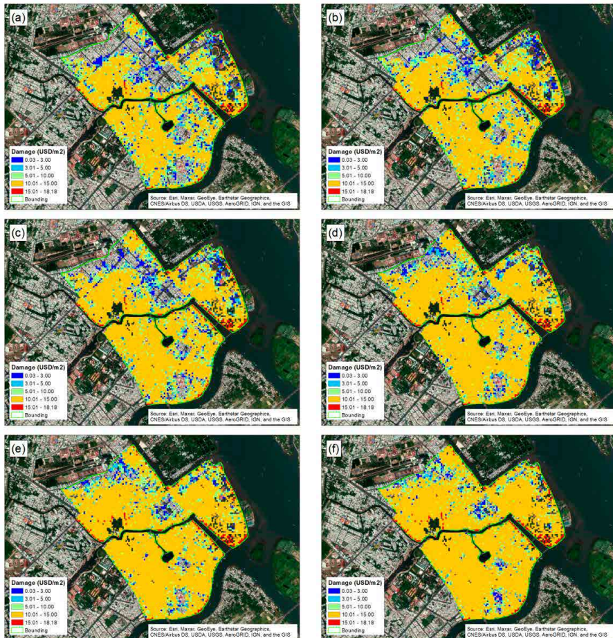
Figure B.4. Flood damage maps for 2050 (scenario #1) corresponding to each return period of water level at Can Tho, (a) 1 yr return period, (b) 2 yr return period, (c) 5 yr return period, (d) 10 yr return period, (e) 20 yr return period, (f) 50 yr return period
