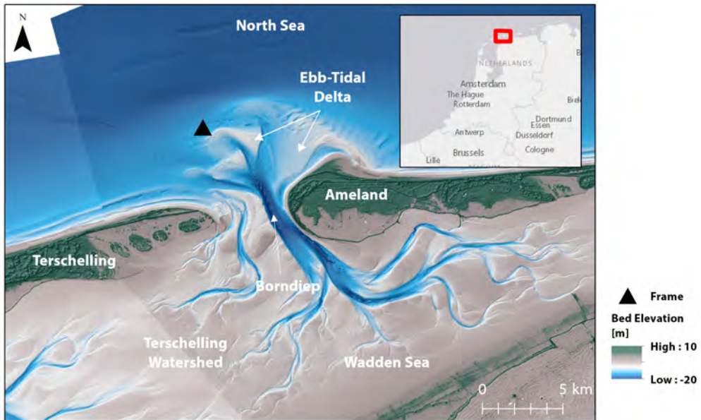
Figure 5.2: Overview of measurements during the September 2017 field measurement campaign at Ameland Inlet, including the frame (AZG-F4) bearing the instruments used in this study. Bathymetry source: Rijkswaterstaat Vaklodgingen. Elevation source: Actueel Hoogtebestand Nederland (AHN), Rijkswaterstaat. Basemap sources: Esri, HERE, Garmin, ©OpenStreetMap contributors, and the GIS user community.
