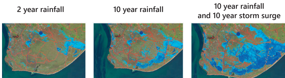
Figure 3-6: flood map for a 2 year rainfall event (left), 10 year rainfall event (middle), and a 10 year rainfall event plus a 10 year coastal surge event (right). Background image: Sentinel-2 (© ESA).
