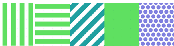
Fig. 6. (Color online) Calibration sample: the color part is electron transparent area and the white is tungsten. Lines: 0.5\ \mu\text{m} wide, 1\ \mu\text{m} pitch; holes: 0.4\ \mu\text{m} diameter, 0.6\ \mu\text{m} pitch.
