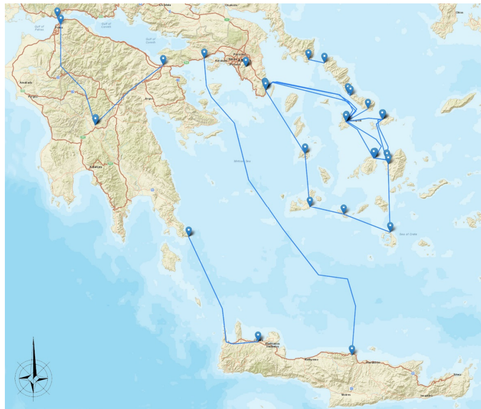
Figure 6. Electrical interconnections already completed or started of the Greek islands with the mainland grid [59].
