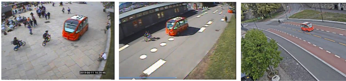
Fig. 4. The different road environments the AV shuttle operates in along the route in Oslo. Left: pedestrian zone, middle: shared space, right: ordinary street with cycle lanes and pavements.
