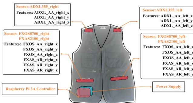
Figure 3.11 The features captured by each sensor and the assembling position of each sensor on the comfort wearable. The same features are captured on the tight-fit wearable, and the sensors are assembled on similar positions.
