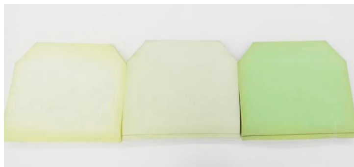
Figure 3.2 Three cushions with different stiffnesses used in this study (A,B,C from left to right)
