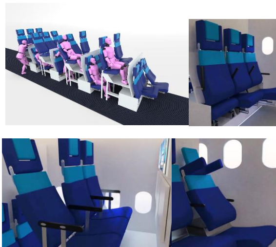
Figure 4.2 The CAD model, upper left: an overview with mannequins, lower left: recline in the upper row, upper right: showing the sliding of the seat pan backwards, lower right: showing the neck rest and recline of the lower seat.
