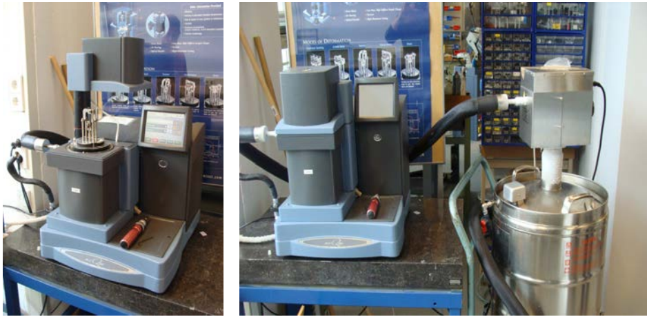
Figure 7.6: Dynamic Mechanical Analyzer Q800 performing the temperature-frequency sweep for a rubber sample designated for PBC belt cover. The liquid nitrogen was used to achieve the temperature inside the testing chamber below the room temperature.
