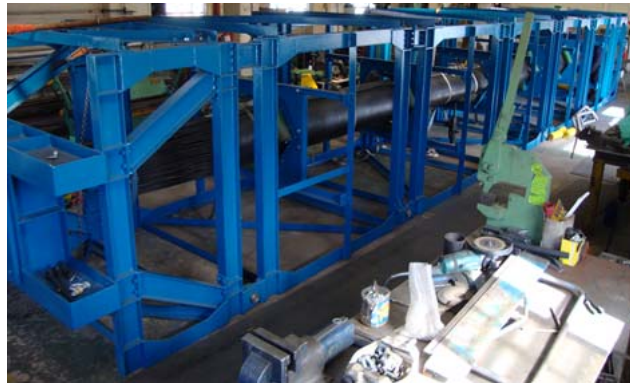
Figure 4.12: Static test rig with frames, assembled by Conveyor Knowledge Information Technology Pty. Ltd (CKIT) in Johannesburg, South Africa, 2010 (Image from Lodewijks and Pang [188]).
