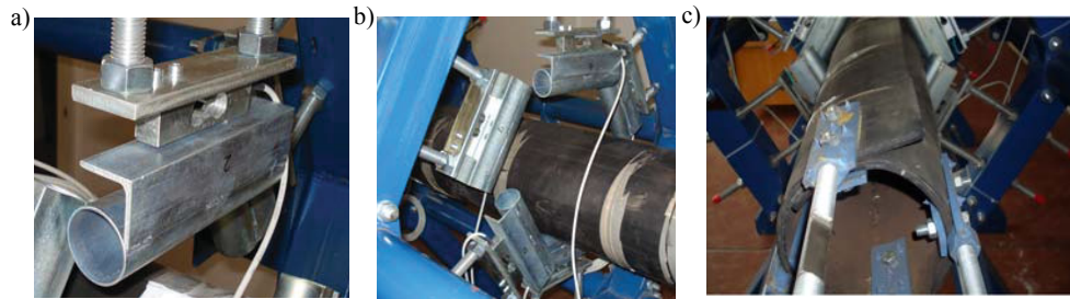
Figure 4.17: Design details of the static test rig, installed in Technical University of Košice in Slovak Republic [155, 162]: a, b) static idler rolls with screw rails (Figures from Michalik and Zajac [155]); c) fixation of a pipe-shaped belt to four plates with the bolt connection (Figure from Molnar et al. [159]).
