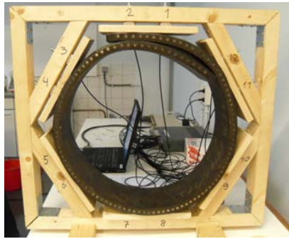
Figure 4.2: Test prototype of a static six-point stiffness device, assembled at Delft University of Technology, Section of Transport Engineering and Logistics, the Netherlands (Figure from [42]).
