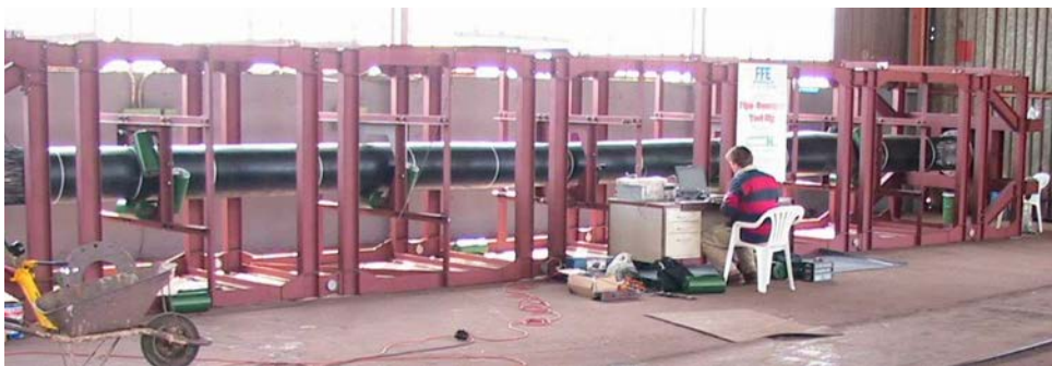
Figure 4.11: Static test rig with frames, assembled by Conveyor Knowledge Information Technology Pty. Ltd (CKIT) in Johannesburg, South Africa, 2005 (Image from [85]).
