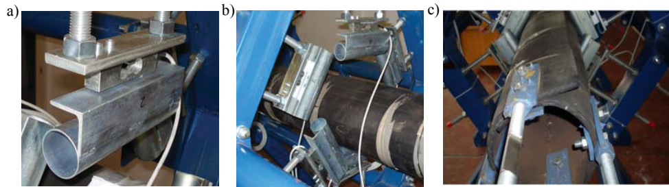
Figure 4.17: Design details of the static test rig, installed in Technical University of Košice in Slovak Republic [155, 162]: a, b) static idler rolls with screw rails (Figures from Michalik and Zajac [155]); c) fixation of a pipe-shaped belt to four plates with the bolt connection (Figure from Molnar et al. [159]).
