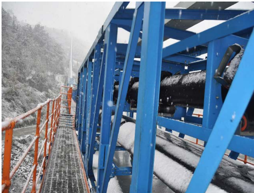
Figure 1.2: Pipe conveyor operating in snow weather condition in Shanxi Province, China (Image courtesy of Zigong Conveying Machine Group Co. Ltd).
