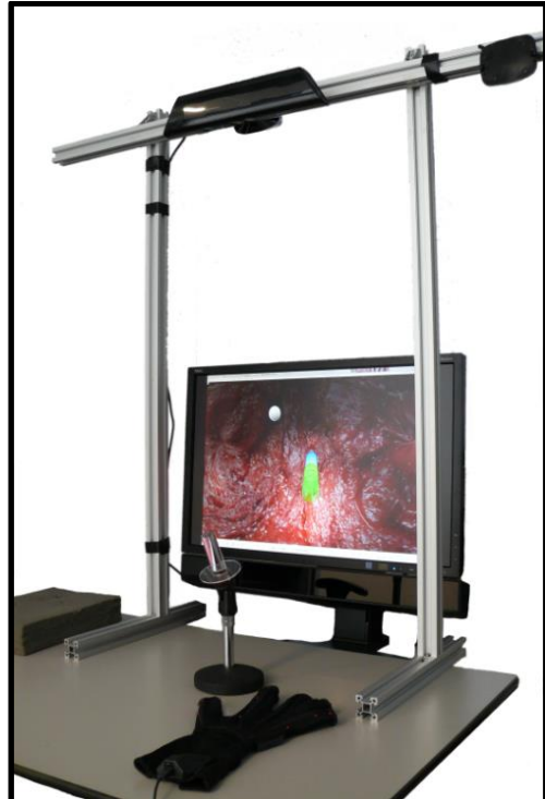
Figure 7.2. Embodiment of the gesture-based design tool. Photograph of the design tool (with the background removed) incorporating a Kinect camera, Nimble VR camera-based hand tracking software, 5DT Data Glove, and custom written C++ software to fuse the sensory information through a Kalman filter to obtain hand postural information.
