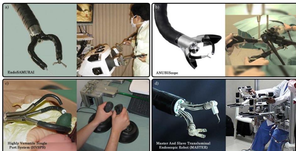
Figure 8.4. Prototyped and evaluated multi-branched systems. a) EndoSAMURAI (Olympus, Tokyo, Japan) [8], b) ANUBIScope (Karl Storz, Tuttlingen, Germany) [9], c) Highly Versatile Single Port System (HVSPS, Can et al. [10]), and d) Master and slave transluminal endoscopic robot (MASTER, Phee et al. [11]). The EndoSamuraï and ANUBIScope are mechanical systems, and the HVSPS and MASTER are both electromechanical systems, relying on master-slave technology. Note that though only a single surgeon is seen at all interfaces, only branch control is truly displayed, with shaft control being negated. In subfigures a) and b) the shaft control handles can be seen to remain unmanned (see black gastroscope handles on top).
