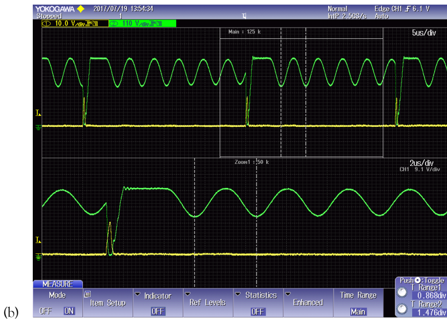
Fig. 5.15. Drain-source voltage V_{ds} and gate voltage V_{gs} for one phase of the IBFC for CH mode: (a) Quasi-resonant operation LVS for V_{ev}=250V , I_{ev}=5A (b) Valley skipping and DCM operation at low powers for V_{ev}=100V , I_{ev}=1A
