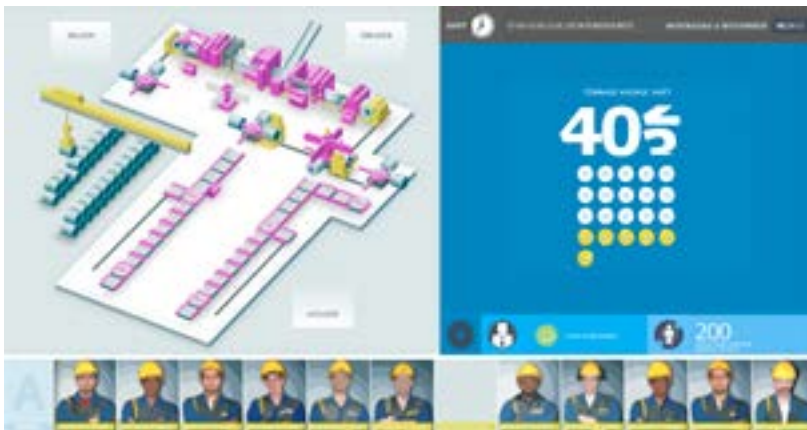
Figure 2.8. Overview page on the new screen at the cutting department: (left) production line, (right) KPI carousel, (bottom) current team.
