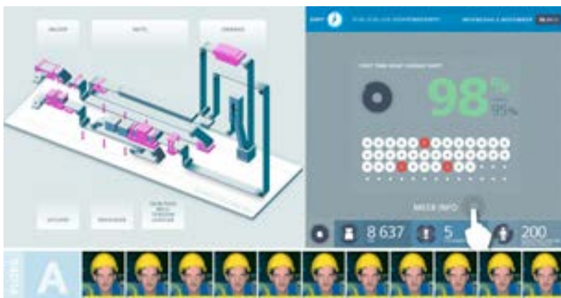
Figure 2.5. Overview page of the screen at the galvanizing department: (left) production line, (right) real-time KPIs, (bottom) current team.
