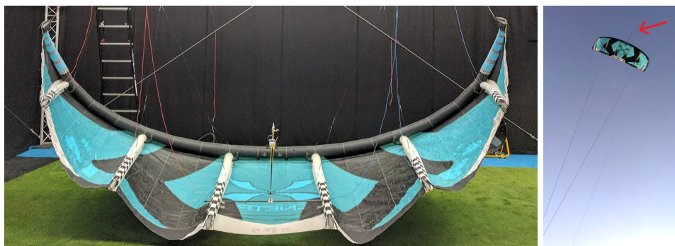
Figure 2. Experimental setup B: Hydra V5 kite with air data boom in the lab and in flight [6].
