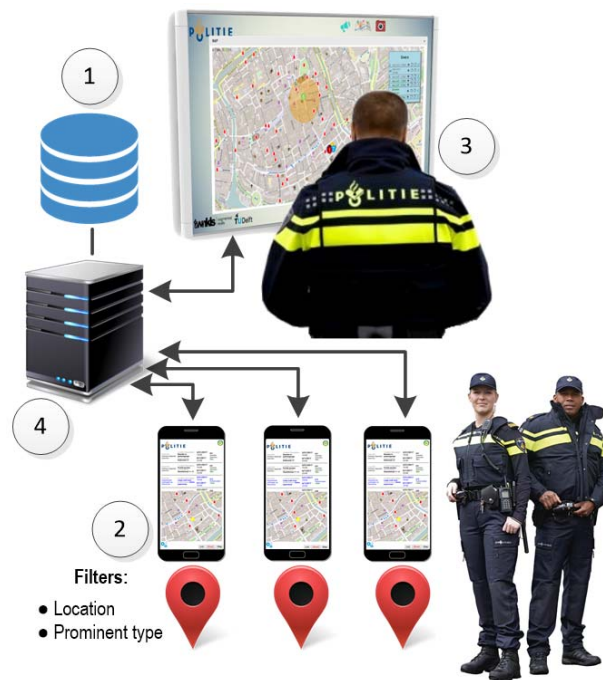
Figure 1: System diagram showing the database system (1), the mobile app for the frontline police officers (2), the user interface for the team leader (3) and the system (back-end) server (4)
