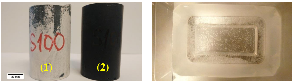
466 Fig. 8a. Pastes S100 at 56 days (left, (1)-unsealed cured sample, (2)-sealed cured sample), the 467 plastic container in which the fluid, condensed on the surface of the specimen S100, was 468 collected after 4 days of unsealed curing (right).
