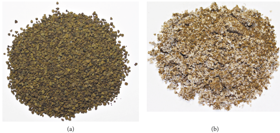
FIGURE 7: \text{MnO}_x/\text{Al}_2\text{O}_3 catalyst after the firing test using neat (a) and gel (b) \text{H}_2\text{O}_2 .
