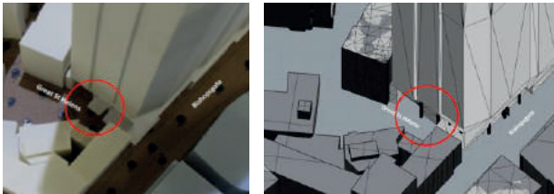
Figure 3. Extra canopy element included in the wind tunnel model (left) and omitted in the CFD model (right)
