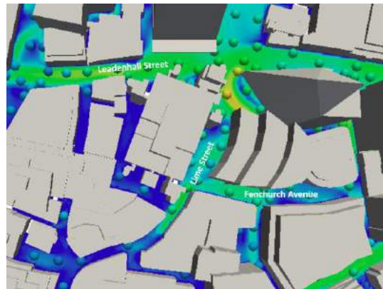
Figure 5. Wind tunnel / CFD comparison (South of the Eastern Cluster). Figure shows mean wind velocity ratio, with wind approaching from 60 degrees
