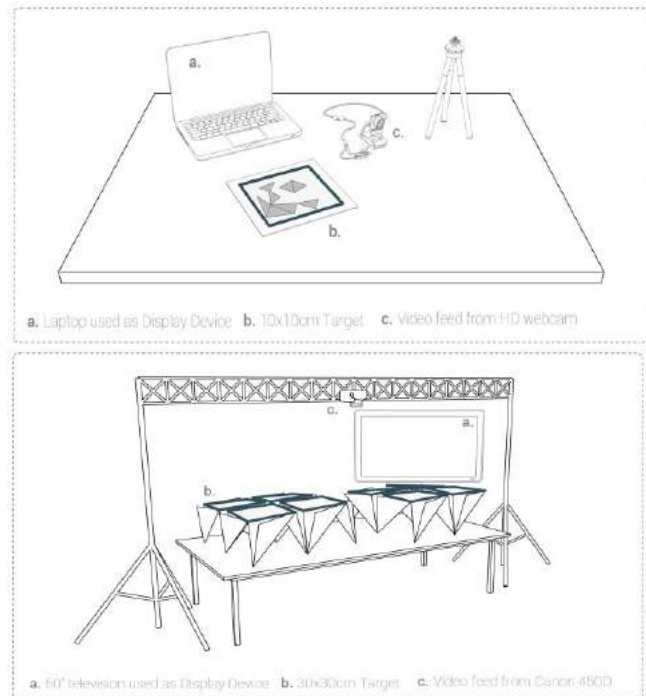
Figure 5. Experiment setup for a 100x120cm test (top) and a 200x200cm test area (bottom).
