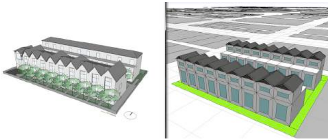
Figure 4. An example conversion of an elementsdb building model (left) to parametric rules in CityEngine (right).
