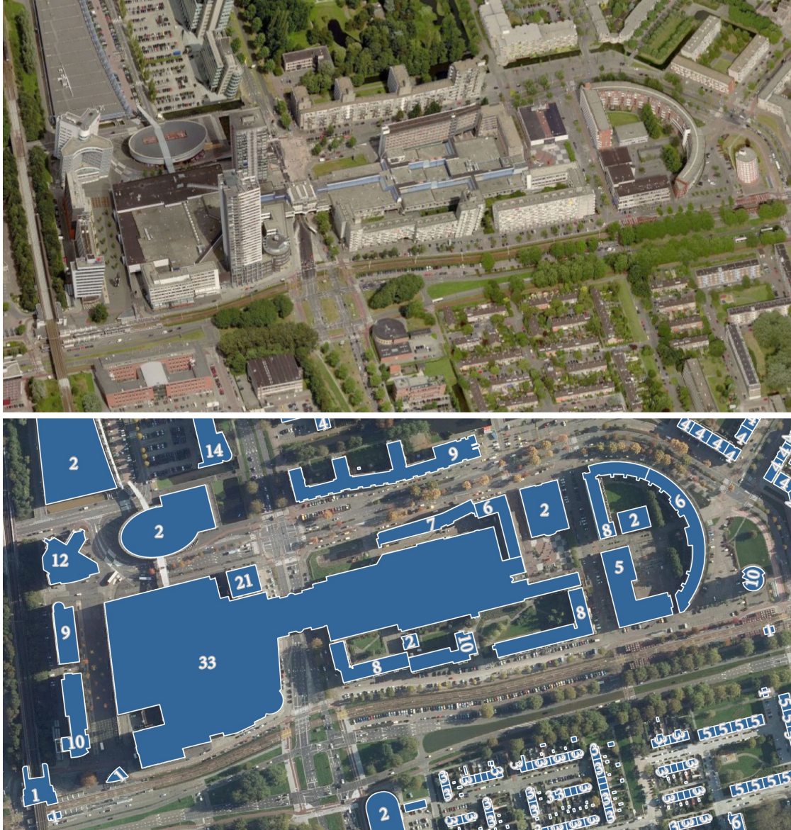
Figure 13: Example of a footprint covering multiple buildings of significantly different heights. The labels represent the number of storeys for each footprint, which we have used to predict heights, and in this case resulted in erroneous predictions. In cases such as this one it is ambiguous to discuss building heights. Footprints (c) Kadaster and City of Rotterdam. Imagery (c) Google and Aerodata International Surveys. Oblique imagery (c) Microsoft and Blom.
