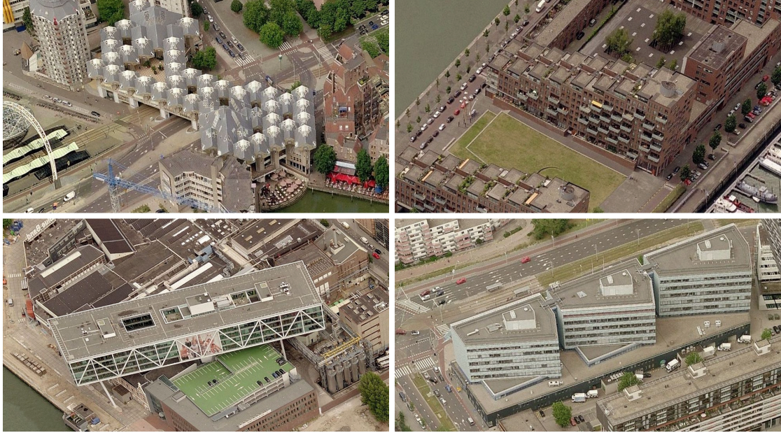
Figure 12: Examples of buildings in Rotterdam with an ambiguous notion of height if extruding the building footprint to a single height was used. Imagery (c) Microsoft and Pictometry International Corp.
