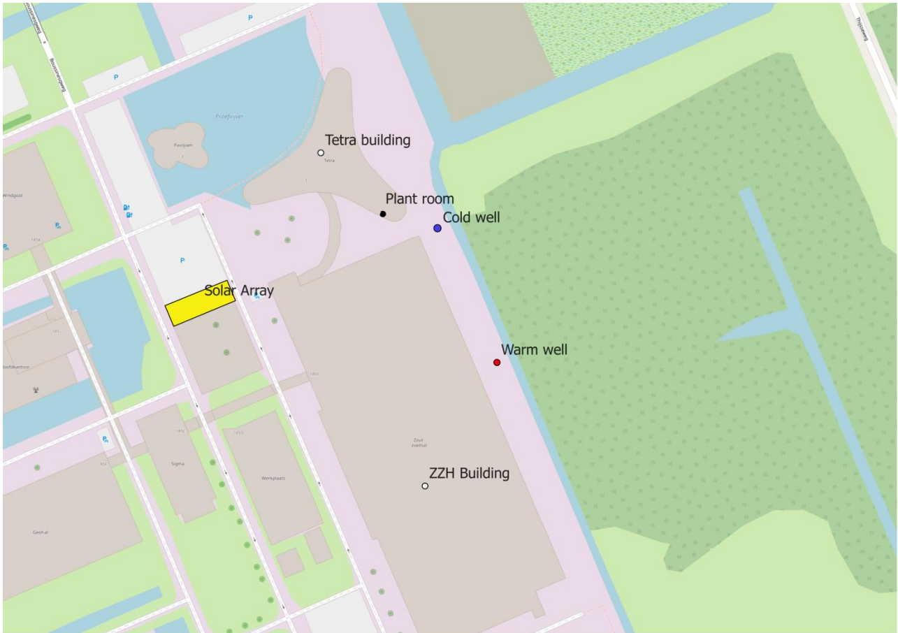
Figure C1. Schematic plan of Deltares campus with the location of different buildings/components indicated.
