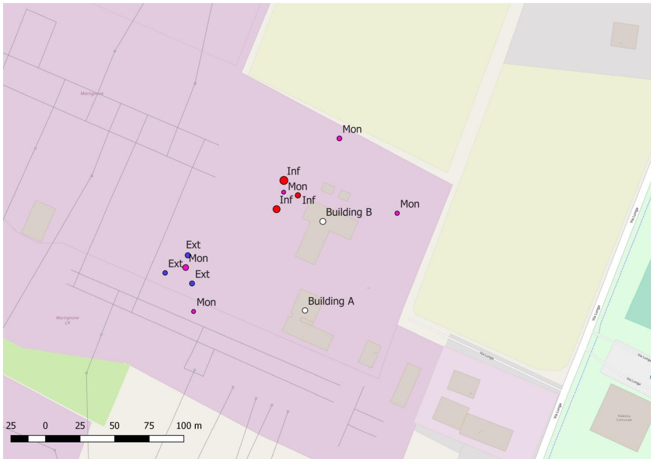
Figure C6. Wells positioning in the Italian pilot plant. Inf= infiltration wells, Ext= extraction wells, Mon = monitoring wells.
