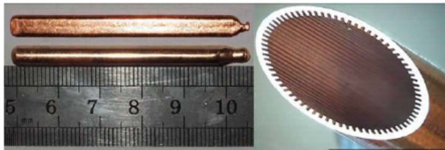
Figure 2. Micro-grooved heat pipe and its grooves [22].
