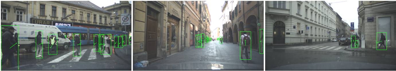
Fig. 8. Qualitative results for orientation estimation. Left and middle image show correct estimations. Right image contains a rare failure case (left person has orientation offset of about 180 degrees)
