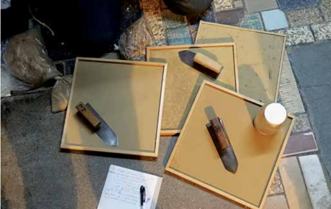
FIG. 21 Different trowels for different surfaces of plaster. The smaller the trowel, the smoother the surface becomes
