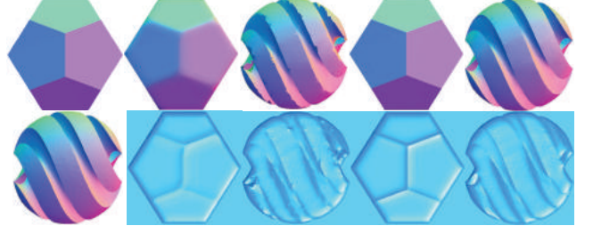
Fig. 6. Using RNF plus GMM can prevent shape distortion of the base surface. The first row shows the original normal map (the first one), the base normal maps obtained by the RNF (the second two) and the GRNF (the last two) respectively; the second row shows the original normal map (the first one) and the bas-relief modeling results from their upper counterparts. Compared to the results by the RNF, the results by the GRNF can better preserve the base’s structures.
